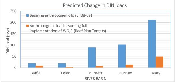
Figure 25 Predicted change in DIN load (t/yr.) assuming full implementation of the WQIP to achieve Reef Plan Targets
